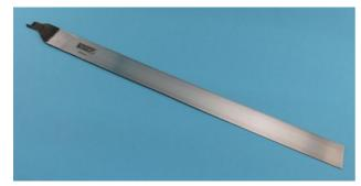
Fitting into a standard reciprocating saw with a ½" tang, the new Spray Foam Insulation Reciprocating Saw Blade measures 19" in overall length with a long 16" cutting length. This double bevel, straight-edged blade is constructed of high carbon steel and is coated with a glazed finish to prevent sticking when cutting foam that has expanded into unwanted areas. The Spray Foam blade and its tang are hardened for long life and improved operator safety in use.
