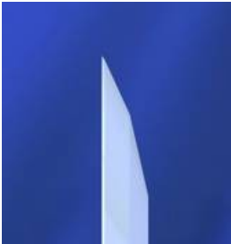
Single Bevel, Compound Angle – two bevel angles – primary and secondary – on one side of the blade only
